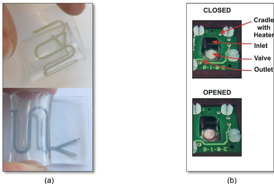
**Figure 1:** (a) Pictures of polyaniline functionalised PDMS chips, acidic on the top and basic on the bottom, as pH sensor. (b) Picture of an ionogel microvalve (7  $\mu$ L) inserted in the holder with integrated heaters at the bottom for fluid control.
